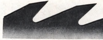
B. FOR EDGER SAWS AND HIGH-SPEED RIPPING.
